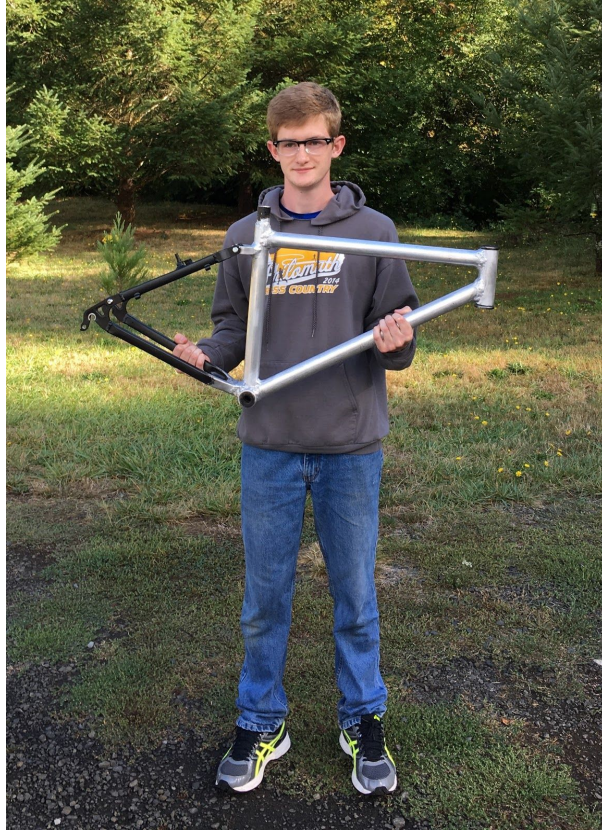
Above: This was just moments after welding the frame together. If you look closely, you can tell I did the welds, since they aren't that great. Below: this is painting the frame with a primer.
